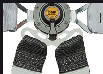
Exclusive double pin T-bar crotch attachment.
